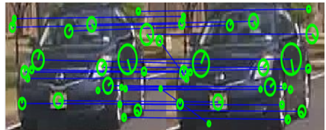
Figure 3: Feature matching between consecutive frames. The images shown above are captured from the bounding boxes.
