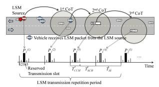
Fig. 5. The overview of ZCOR in multi-hop LSM dissemination;  $P_i^{(j)}$  is jth hop LSM packet with a sequence number i.
