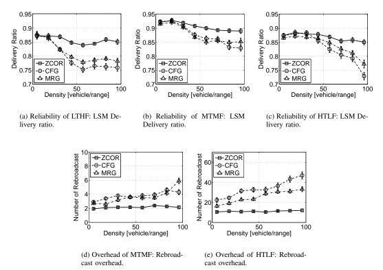
Fig. 13. Reliability and overhead under various vehicle density conditions.
