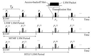
Fig. 6. Transmission slot reservation in each class of LSMs (L=5); MTMF geocast has 2-hop range (h=2).
