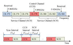
Fig. 3. Multi-channel structure in WAVE standards.
