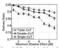
Fig. 15. Gains from multi-CoT against shadow fading; vehicle density is 55 [vehicle/coverage].
