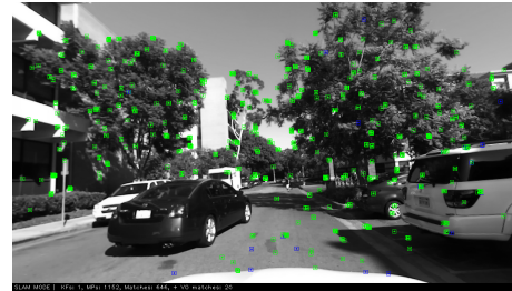
Figure 4—The green dots represent static features that are used to construct the sparse HD map, while features from the moving vehicle are filtered out.
