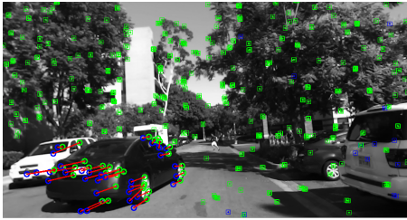
Figure 6 —Estimating the motion of a vehicle. The lines show the motion of features (represented by circles) across two successive frames.
