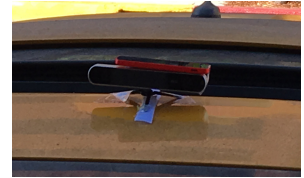
Figure 6 —ZED Mounted on top of the Windshield with Smartphone Attached
