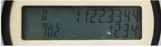
**Figure 5: Spoofing attack validation: The LED display of the ERT reader received the spoofed packet with an ID of 11223344 and data reading of 1234.**
