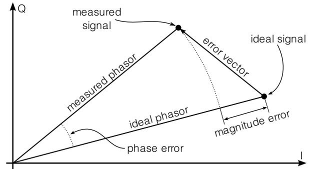
Figure 5: Modulation errors
