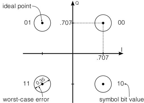
Figure 4: The 4 symbols of QPSK on I/Q plane
