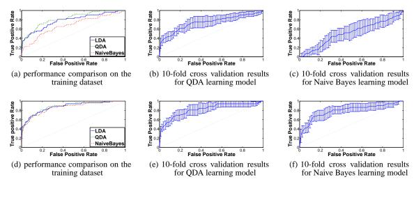
Figure 9: Detecting truck from automobiles with manual feature selection
