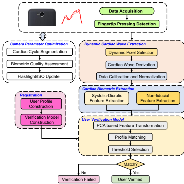
Figure 4: System Overview of CardioCam.
