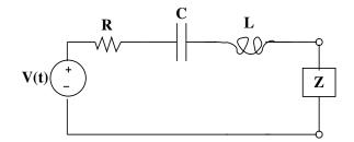
Assume sinusoidal steady state operation at some frequency  $\omega$ .
