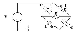
(a) (2 pt) Assume  $V = Ve^{j\theta}$  and  $I = Ie^{j\theta}$ . What is the amplitude of the voltage across the resistor?
