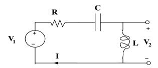
Assume sinusoidal steady state operation at some frequency  $\omega$  and suppose  $\mathbf{V}_1 = V e^{j\theta}$  and  $\mathbf{I} = I e^{j\phi}$ .
